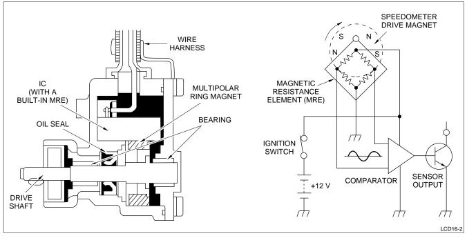
Figure 2. MRE Vehicle Speed Sensor and Supporting Circuitry (Toyota)
