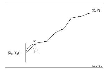
Figure 9. Vehicle Positioning by Vector Summation
