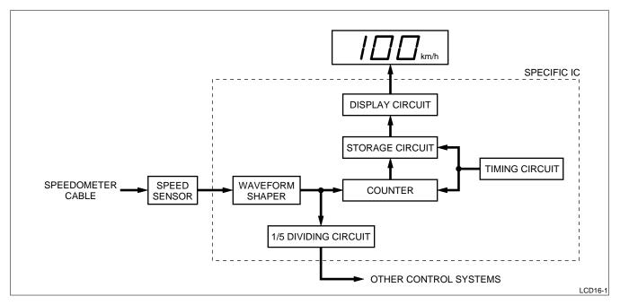
Figure 1. Systems Layout of a Typical Speedometer
