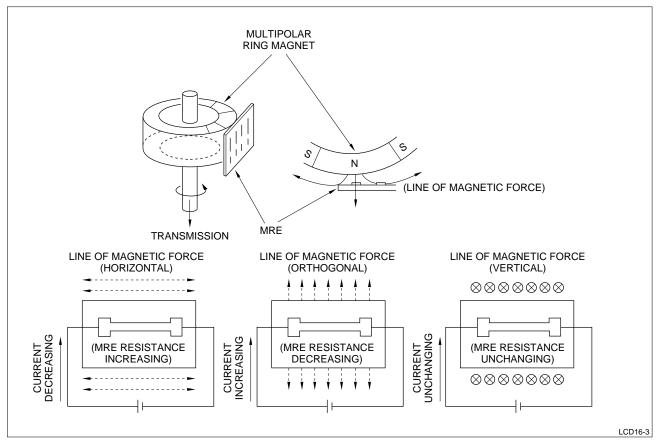
Figure 3. Operating Principle of MRE
