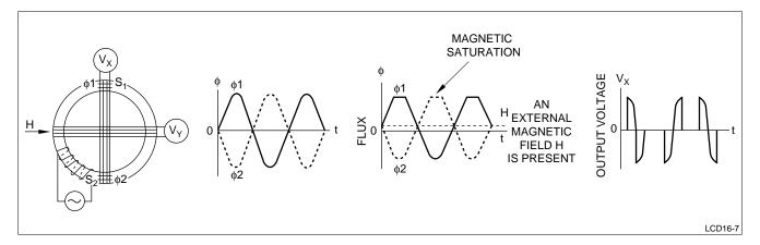
Figure 7. Basic Compass Operation Principles and Output Voltage Waveforms
