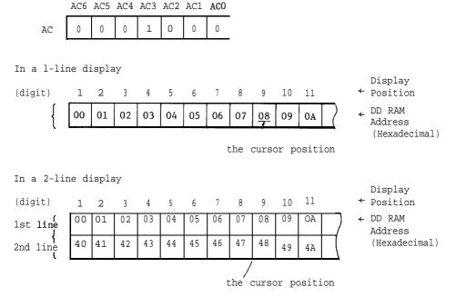
(Note) The cursor or blink appears when the address counter (AC) selects the character generator RAM (CG RAM). But the cursor and blink are meaningless.
